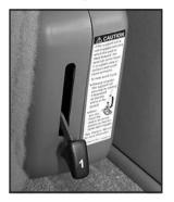
1. To return the seatback to an upright position, pull up on the release lever labeled 1 and then pull up on the seatback until it locks into the upright position.
